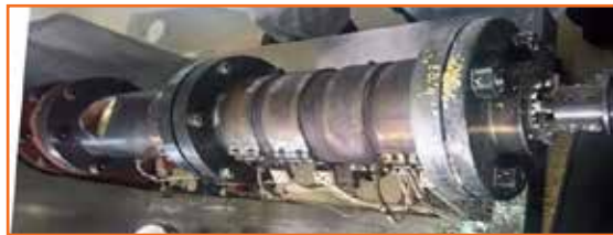
Fig 5.2.18 Heating/cooling section in extruder machine
