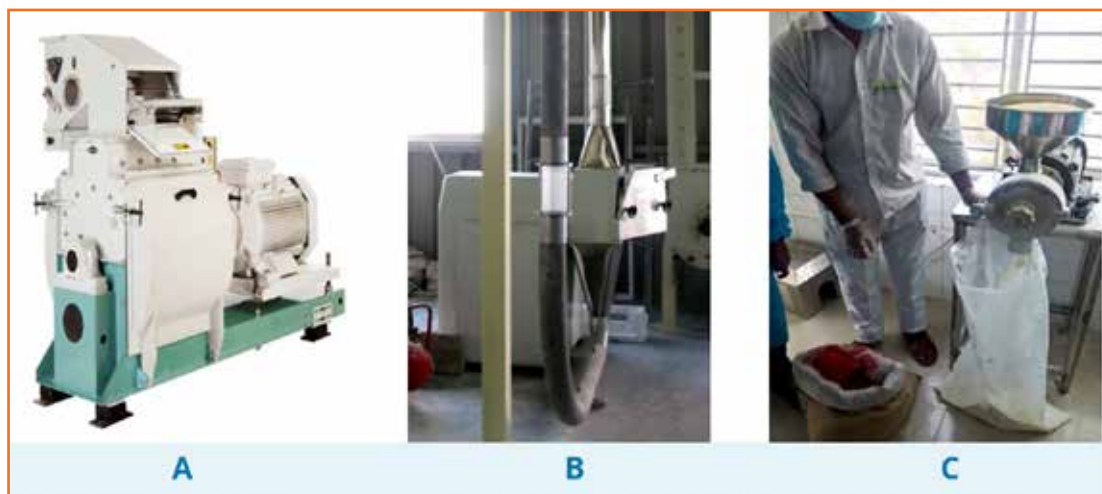
Fig 5.2.3 Different types of mills. (A) Hammermill with up to 2000kg/h, (B) Hammermill with up to 300kg/h in automated production, (C) Small Diskmill with manual operation
